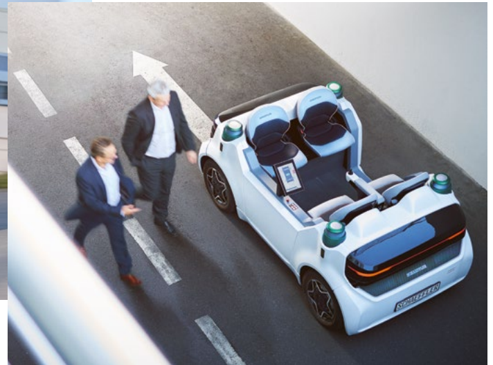
The Schaeffler Mover is a platform for developing autonomous driving technologies.
